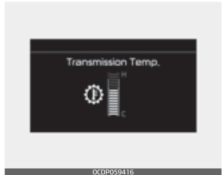
This mode displays the transmission temperature.
