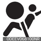
The purpose of the air bag warning light in your instrument panel is to alert you of a potential problem with your air bag – Supplemental Restraint System (SRS).
