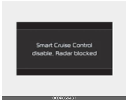
If the radar or cover is dirty or obscured with foreign matter such as snow, this message will appear and it will disappear after for a while.
