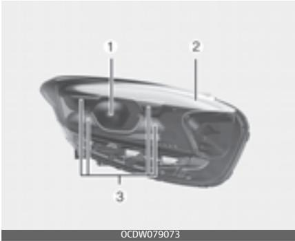
If the Low/High beam lamp(1), Front turn signal lamp(2), Day time running lamp/Position lamp(3) does not operate, have your vehicle checked by a professional workshop.
