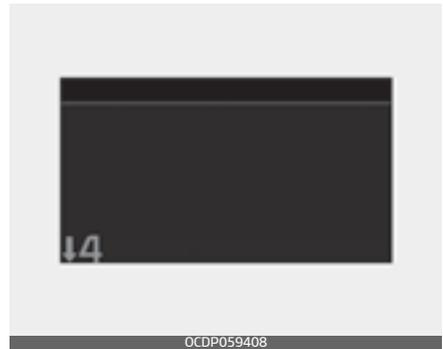
In the Manual shift mode, this indicator informs which gear is desired while driving to save fuel.
